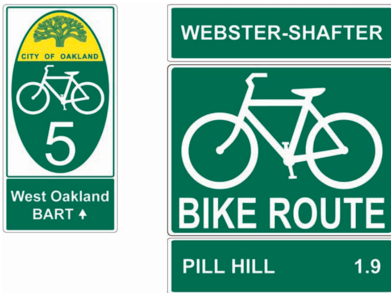
Figure 3.1: Bicycle Wayfinding Signage . Wayfinding signs for bicyclists include the “Bicycle Route Number Marker” sign (left) and the “Bike Route” sign (right), shown here with supplementary placards for the bikeway name and a destination along the route. The relative size of the signs in this illustration reflects that of typical installations in Oakland.
