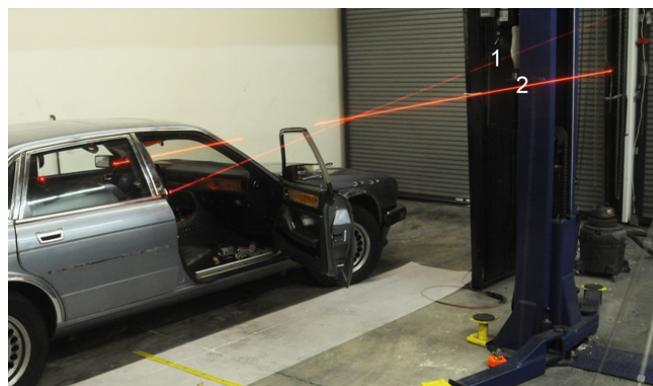
**Figure 4:** 1- laser on trajectory rod inside the vehicle. 2- laser mounted on a tripod outside the vehicle.
