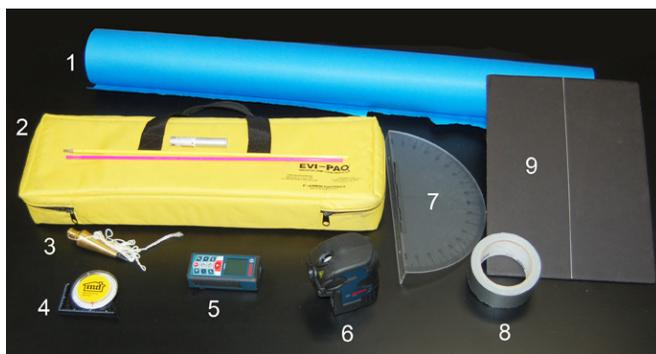
**Figure 1:** 1- butcher paper, 2- laser trajectory kit, 3- plumb bob, 4- inclinometer, 5- electronic inclinometer, 6- laser plumb bob, 7- zero edge protractor, 8- duct tape, 9- card.
