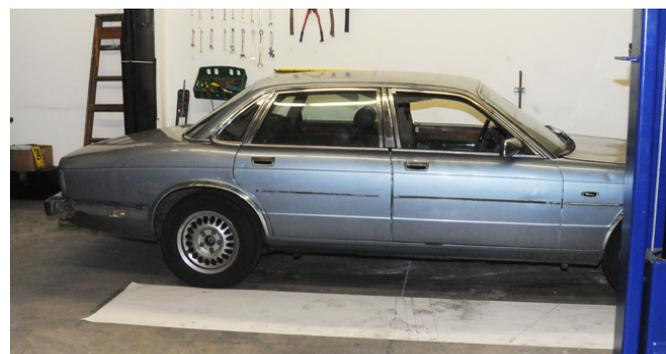
**Figure 2:** Butcher paper aligned parallel to vehicle side and taped down
